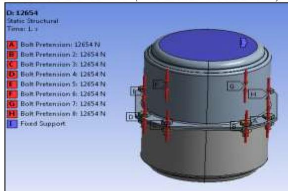
**Fig.8;** Boundary condition for load 90 %
