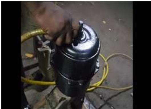
**Fig.3:** compressed air filling in oil sump
