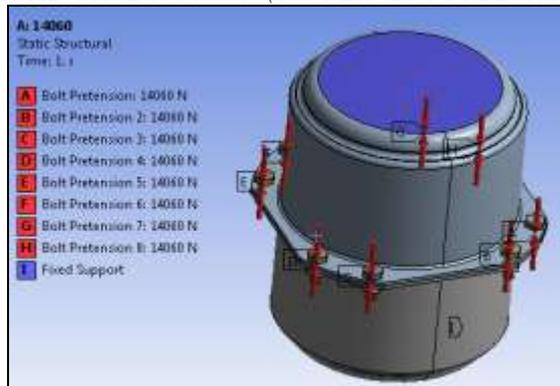
**Fig.7;** Boundary condition for load 100 %
