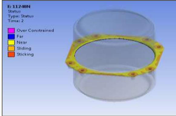
Fig.27; Contact status at 80 % load
