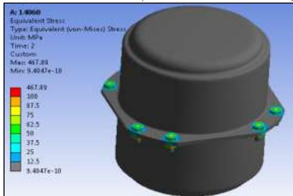
Fig.19; VON MISES Stress at 100 % load
