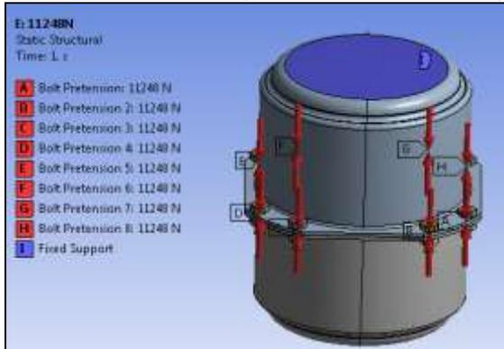
Fig.9; Boundary condition for load 80 %
