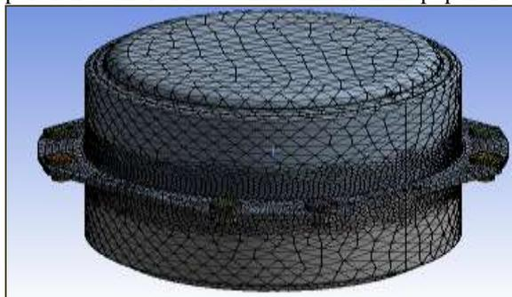
**Fig 6:** Discretization of specimen
