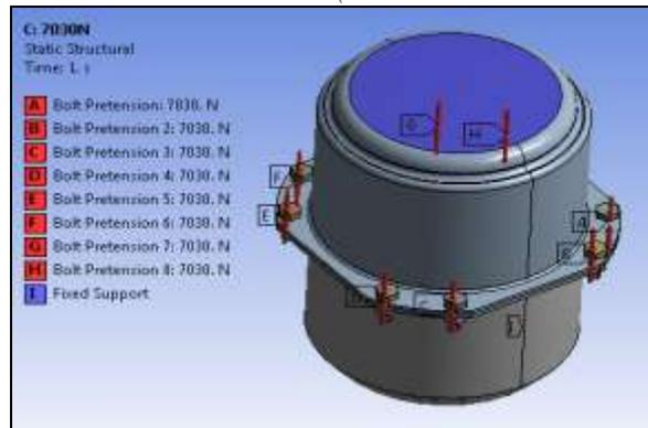
Fig.12; Boundary condition for load 50 %
