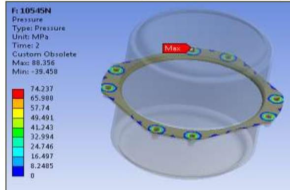
Fig.34; Contact pressure at 75 % load
