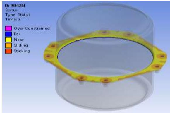
Fig.29; Contact status at 70 % load
