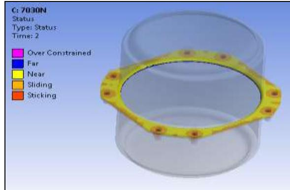
Fig.30; Contact status at 50 % load
