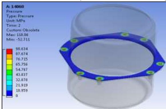
Fig.31; Contact pressure at 100 % load
