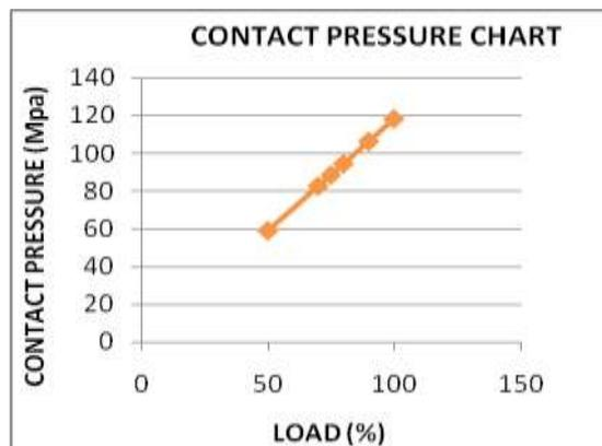
Graph 3: Contact pressure induced at three loads in FEA
