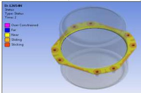
Fig.25; Contact status at 100 % load
