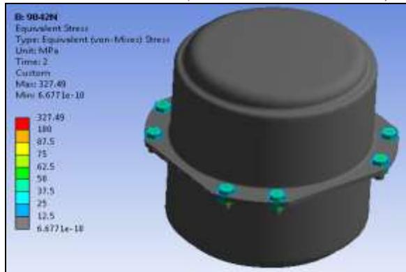
Fig.23; VON MISES Stress at 70 % load
