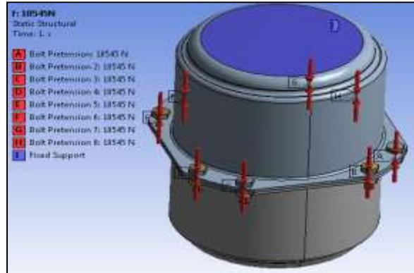
Fig.10; Boundary condition for load 75 %
