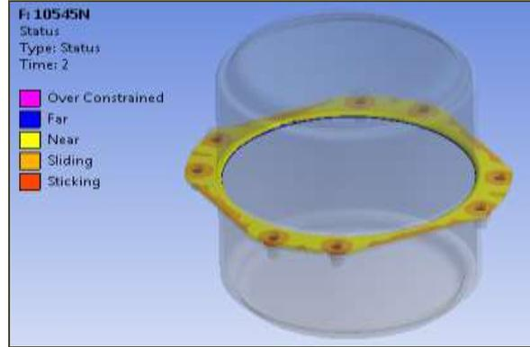
Fig.28; Contact status at 75 % load
