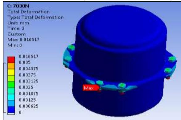
Fig.18; Deformation in 50 % load
