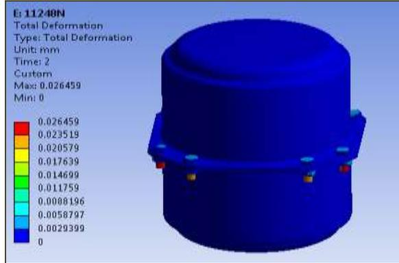
Fig.15; Deformation in 80 % load
