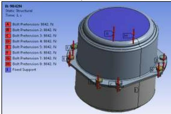
Fig.11; Boundary condition for load 70 %
