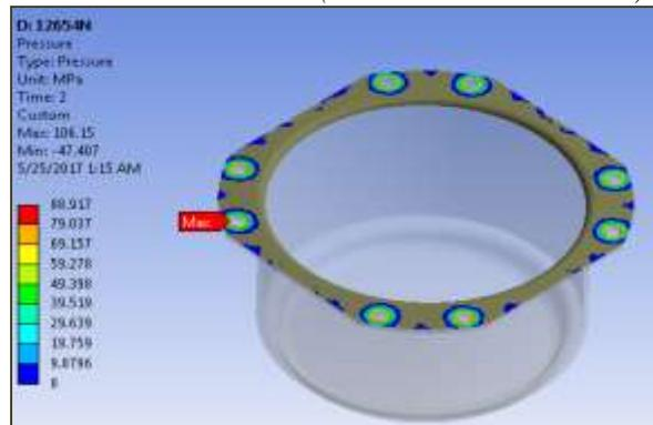
Fig.32; Contact pressure at 90 % load
