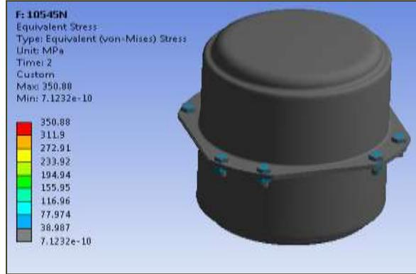
Fig.22; VON MISES Stress at 75 % load
