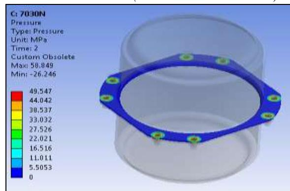
Fig.36; Contact pressure at 50 % load
