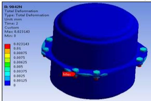
Fig.17; Deformation in 70 % load
