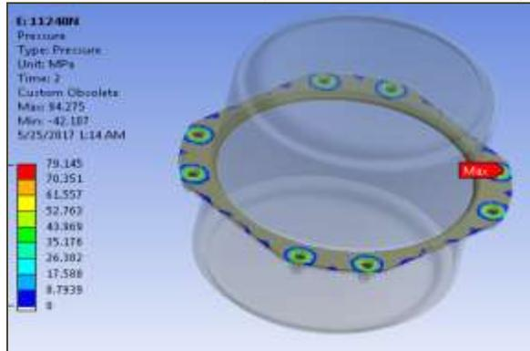
Fig.33; Contact pressure at 80 % load
