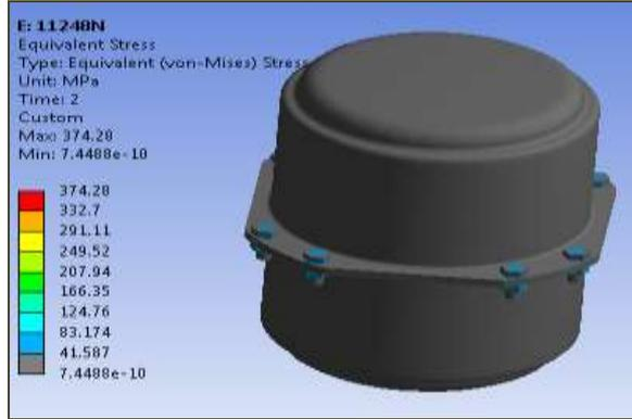
Fig.21; VON MISES Stress at 80 % load
